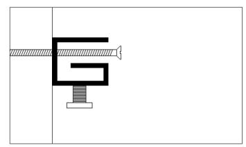
Once you have drilled ALL holes, place the plastic raw plug into the hole, and screw in all screws tightly.
