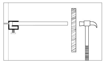
If you can't manage to push the glass completely in, get some wood and a hammer or mallet. Place the wood at the front of the glass and tap it with the hammer or tap directly with the mallet.
