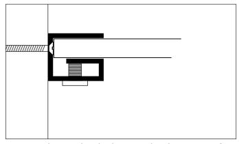
Now tighten the bolts on the bottom of the braket to secure the shelf. This system is designed to be used with **Toughened Glass** ONLY!
