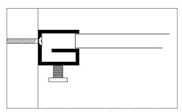
Once the bracket is installed, place the glass into the front of the bracket and by hand, push it in as far as you can.
